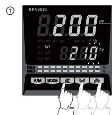
Press any key among the **↖, ↻, ▲, ▼** in RUN mode to enter into SV setting mode. Last digit (100 digit) on SV display part flashes.
