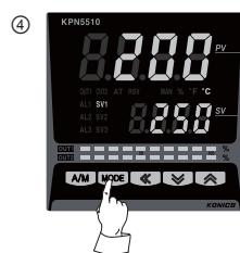
Press the **MODE** key to save the setting value. If there is no additional key operations in 3 sec., the changed SV is automatically saved.
